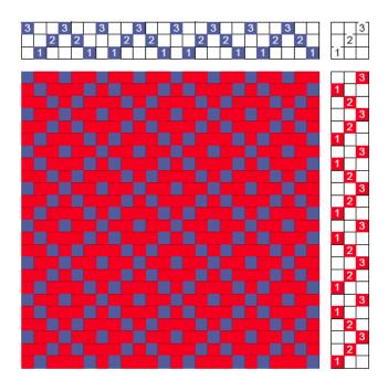
The drawdown is above. As any other structure woven on an odd number of shafts, the fabric is unbalanced: one side is west dominant, the other warp dominant. The drawdown is for a rising
