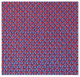
shed loom; one shed is raised at a time, leaving the weft to cover the threads on the other two shafts that did not rise.
